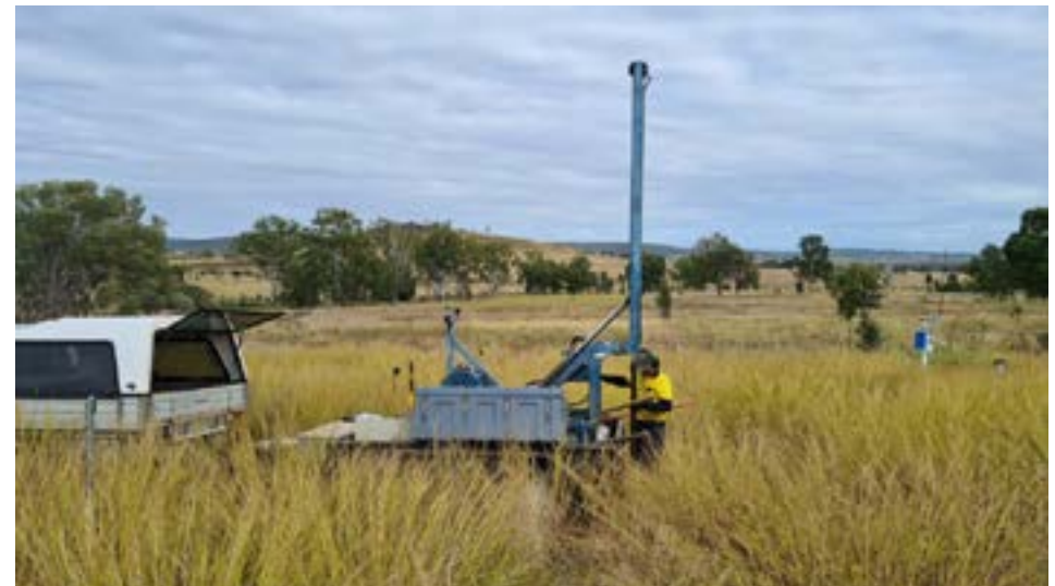
Baseline soil sampling using a hydraulic rig
