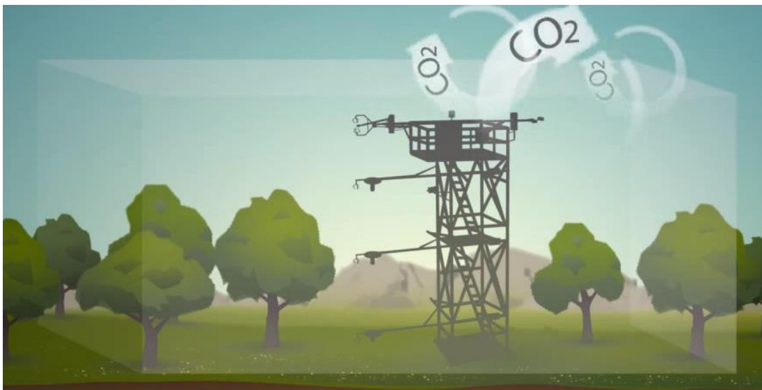
Figure 2: The measurement 'box' of the flux tower measuring CO 2 entering and leaving a defined area (Source: LICOR user manual)
